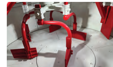
Rotating case with counter-rotating mixing star
