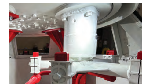
Planetary gearbox sealed to reduce maintenance and prolong life
