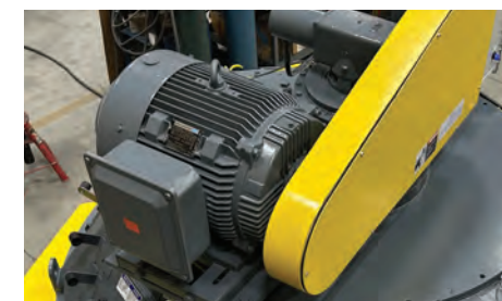
Top-mounted motor is totally enclosed for dust protection
