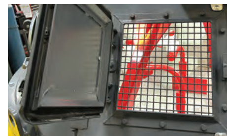
Hinged access door with inspection hatch
