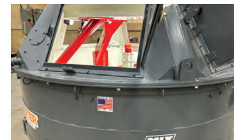
Heavy-duty mixer tank structure and cover assembly with top-mounted drive
