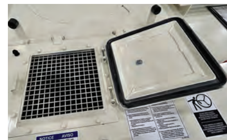
Hinged inspection door on mixer cover
