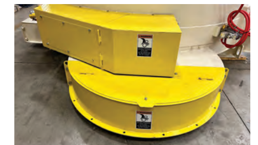
Mixer discharge door with guarding and round connection flange
