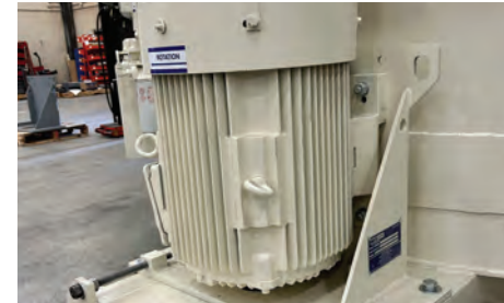
Mixer high-efficiency motor with protective dust shield
