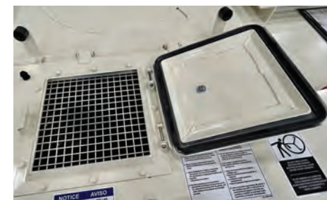
Hinged inspection door on mixer cover
