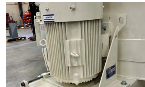
Mixer high-efficiency motor with protective dust shield
