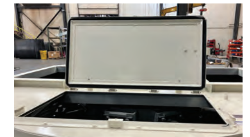
Hinged access doors for cleaning & part replacement
