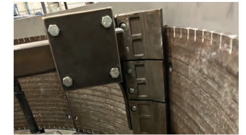
Cast Ni-Hard wall scrapers; optional MAXALLOY scrapers are available
