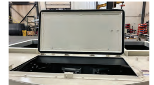
Hinged access doors for cleaning & part replacement
