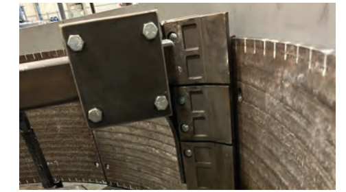
Cast Ni-Hard wall scrapers
