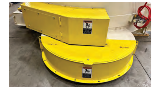
Mixer discharge door with guarding and round connection flange
