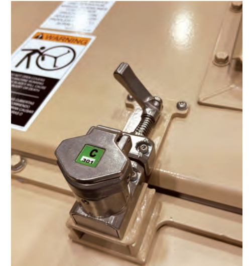
Hinged access door trapped key interlocks
