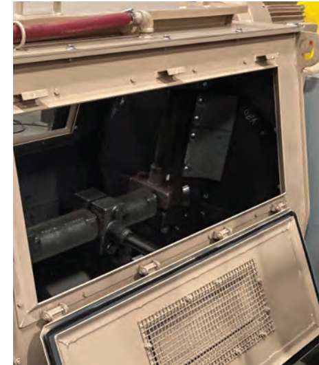
Steel, dust-tight gasketed access door
