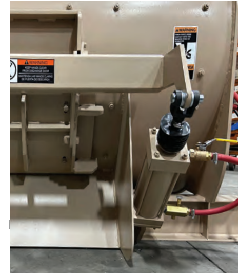
Pneumatically operated discharge door for fast discharge
