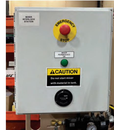
Mixer interlock controls protect personnel from exposure to moving parts
