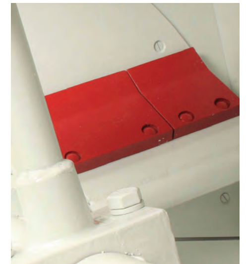
Cast Ni-Hard wall scraper blades resist wear*
