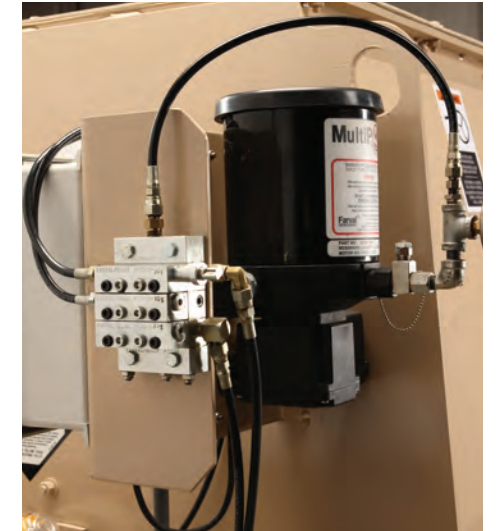
Shaft seal lubrication system
