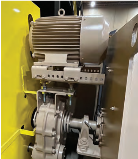
Shaft mounted mixer drive with oil-bath lubricated gear box for long life
