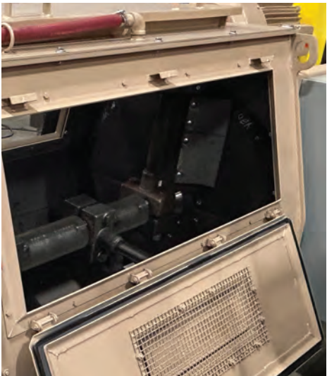
Steel, dust-tight gasketed access door
