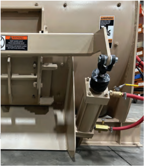
Pneumatically operated discharge door for fast discharge
