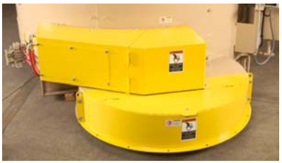
Discharge Door Oversize discharge door assures, fast clean discharging of material. The door guard is hinged and provided with an inspection hatch. The door slides in a protected track to maintain positive closing, regardless of the mix.
